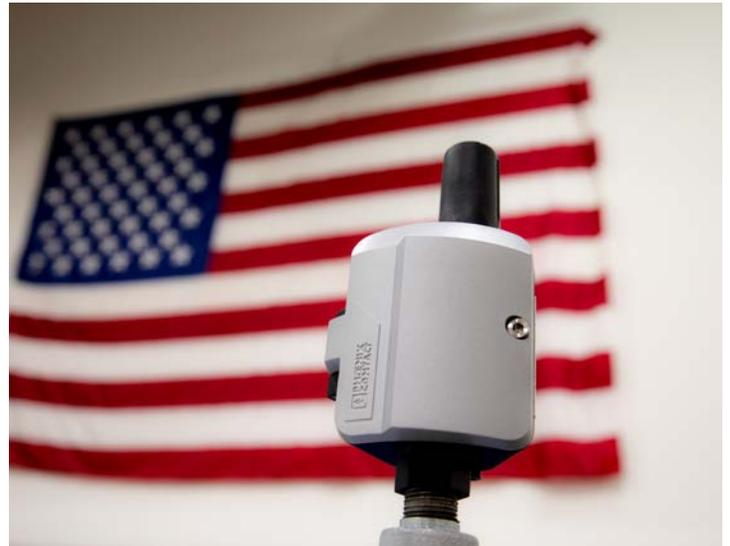
**Figure 2: The WirelessHART transmitter makes it easy to access critical data without the cost of running Ethernet cables to the remote sites.**
